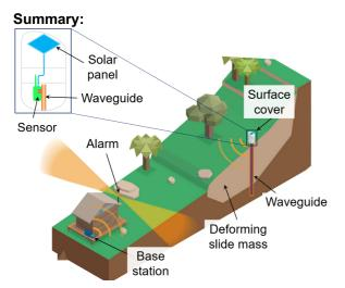
There is an urgent need for improved and affordable approaches for health monitoring of geotechnical infrastructure systems to facilitate asset management (e.g. slopes, foundations, dams and buried pipes). A proportion of energy dissipated during deformation of soil, soil-structural interactions and seepage processes is converted to heat and sound. The high-frequency (>10kHz) component of this sound energy is called acoustic emission (AE).
